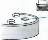
Replace access plug or install an inverted, screened well vent if one is not present. Silicone (or any other caulking) is not an acceptable permanent fix for any well opening deficiencies.
