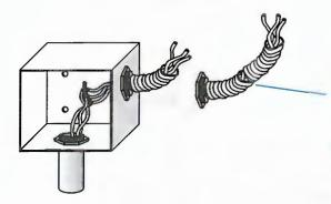
An electrical junction box shall be watertight (including at box attachment to the well casing and electrical conduits attached to the box) to prevent contaminants from entering the well. Replace damaged flexible conduit.
